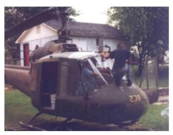
Windshields, both left and right hand to fill the void, took three sets of hands to install. Don Head pearched on the nose for several hours while we installed the hundreds of nuts and bolts...
