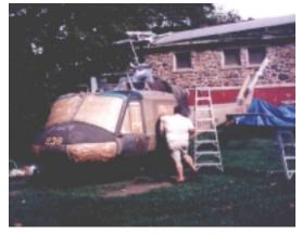
Masking off was an important part of the preparations prior to the first touch of the painter's hand...
